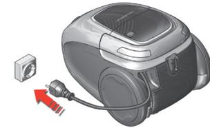
**6. Pull out the power cord and plug it into the mains.** A zero "0" will be visible in the display on the body.
