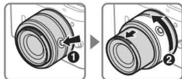
To unlock the zoom ring and extend the lens for use, press the retractable lens barrel button (1) and rotate the zoom ring in the direction shown in Figure 2. The lens can be retracted and the zoom ring locked by pressing the retractable lens barrel button and rotating the zoom ring in the opposite direction.
