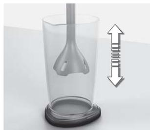
3. **Insert the stick mixer deep into the beaker**, begin mixing by starting at normal speed. Make sure the beaker is no more than 2/3 full. If you do not use the beaker, do not immerse the mixing foot more than 2/3 of its length. Move stick mixer lightly up and down to ensure best processing of content. Release switch to stop.
